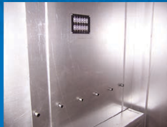
Interior Thermocouple Jack Panel & Vacuum Stubs
