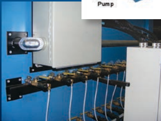
Vacuum Lines for Composite Bag Applications
