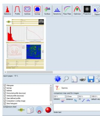
for evaluation and comparison. That is, the measured dose map must be projected to the grid of the plan. To do this FilmQA Pro™ software generates a projection map, i.e., the measured dose map is recalculated by averaging individual pixels values grouped to reproduce the spatial resolution of the
