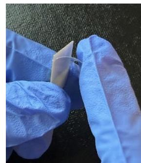
figure 2-3 peeling adhesive cover method
