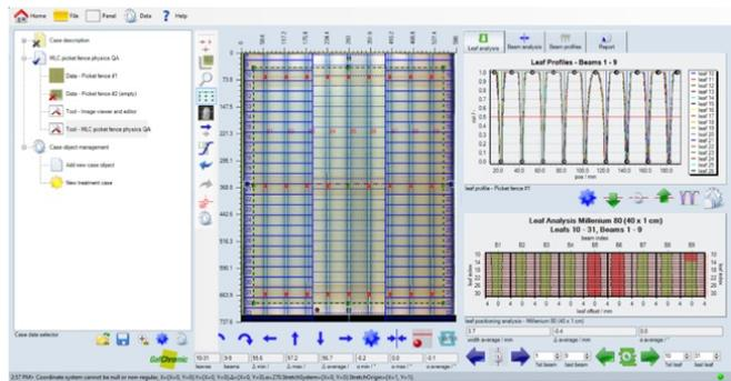
Adjustments are complete when the leaf borders on the film line up with the overlaid MLC leaf borders (solid blue lines, dotted blue line are leaf center lines). The space around the leaf center line is used to create profiles to detect the leaf openings as extrema. Select the "Leaf Analysis" tab to commence the analysis.
