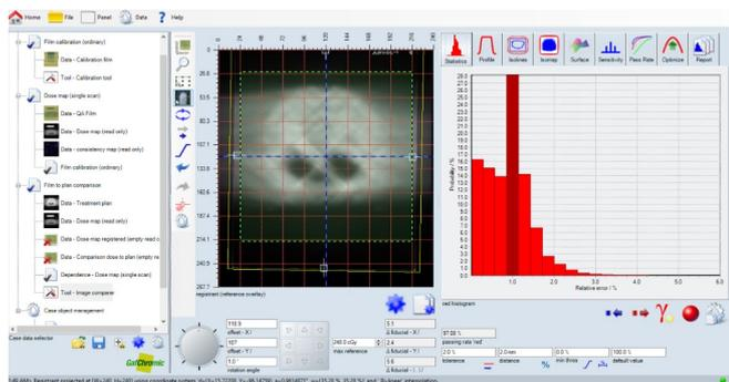
In the example case the gamma test passing rate is  $>95\%$  for 2% dose tolerance at 2 mm. Passing rates  $>95\%$  for the 2%/2 mm criteria are common with film evaluation, but with passing rates that high, there is little sensitivity in using the passing rate to search for a more optimal fit while using the coarse 2%/2 mm evaluation criteria.
