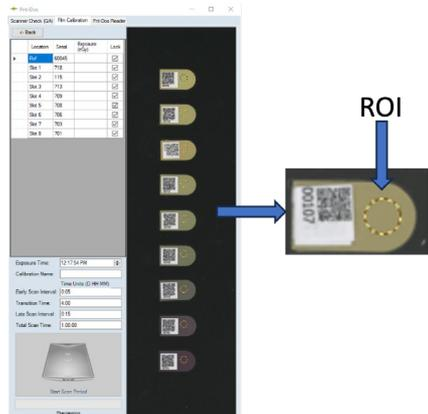
**note:** If an ROI circle does NOT appear on a Pnt-Dos™ device click on the “Back” button above the calibration table, open the lid to the scanner and ensure the Pnt-Dos™ devices are seated well by gently pushing down on the white or adhesive side of the device, then rescan.
