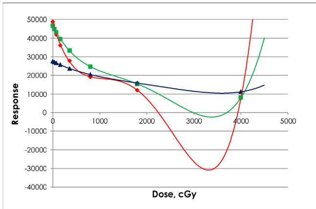
The benefit of using the type of rational function described above is that the user can reduce the number of dose points required for calibration. Figure 3 shows the fit when four of the data points were removed. It is almost identical to the fit in Figure 1 with seven data points. The function has three constants  $a$ ,  $b$ , and  $c$  and is fully defined with three data points – two films exposed to known doses plus one unexposed film.
