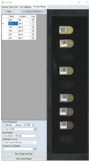
**note:** If the ROI circle does not appear on the exposed Pnt-Dos™ devices, click on the “back” button, open the lid, and carefully reseal the devices or gently press on the white or adhesive side to ensure the devices are flat on the scanner glass plate, then rescan.
