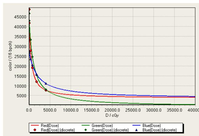
Contrast this to the behavior when the same data is fitted to polynomial functions (in this case 4th order) as shown in Figure 2. Obviously, the polynomial functions don’t behave like film – film doesn’t get lighter in color and more transparent at high doses. Also, polynomial functions are unacceptable because they oscillate between dose values. The fit with the polynomial function could be improved with additional dose points, but it takes more time and doesn’t address the fundamental problem.
