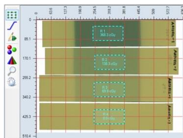
Use the Frame Selector tool to draw areas of interest in the center of each strip. A frame can be easily duplicated by holding down the "Control" key and pointing/clicking with the mouse. Calibration
