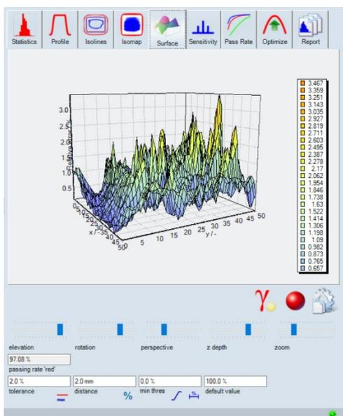
The Projection Map is critical to the proper calculation of the dose distribution comparison functions. The dose map and treatment plan cannot be compared without placing them in the same spatial domain. Because film is usually scanned at  $\geq 72$  dpi or more, the spatial resolution of the dose map is almost always much greater than the
