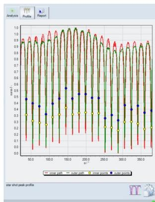
Profiling along the analysis path verifies the quality of the detected intersection points between the beam lines and analysis circles. The Star Shot Peak Profile (left) shows the color channel values along both analysis path circles and the locations of the detected beam line points (minima when darker otherwise maxima).
