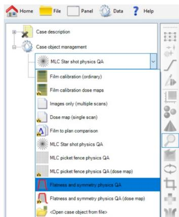
Click on “Add New Case Object” under the “Case Object Management” heading. A drop-down menu will appear and gives the user several options. Select “Flatness and Symmetry Physics QA” (Shown left). There are two types of objects to select: ‘Flatness and Symmetry Physics QA’ (Shown left) can hold any number of
