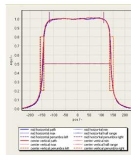
The maximum or CAX value can be normalized between 0 and 1. If the base line of the profile is disturbed (left and right values are different), the base line can
