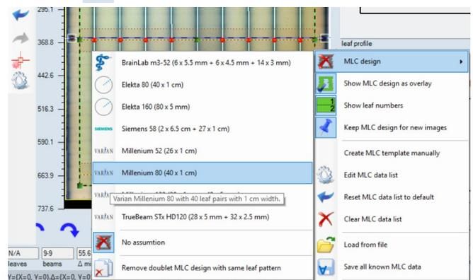
If the targeted MLC design is not available, then use "Create MLC Template Manually" to input new data. When the MLC design is selected, the overlay is displayed in the
