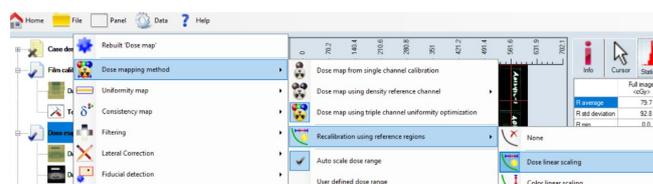
Display the new dose map in the Image Window and look at the values in the Statistics table. The exposed reference film is now exactly 313 cGy in each color channel. For the unexposed film the tabulated values are not exactly zero, but only because FilmQA Pro™ doesn’t display negative dose values. Any negative calculated value is set to zero as shown by the histogram.
