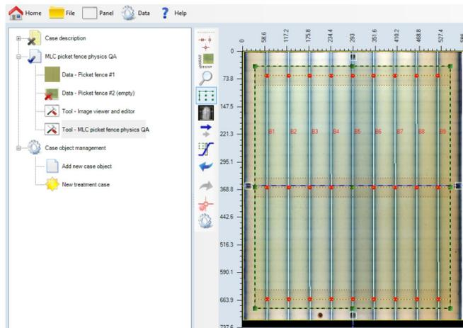
The isocenter (blue/black dashed lines) is automatically fitted to the marked fiducials as shown right.
