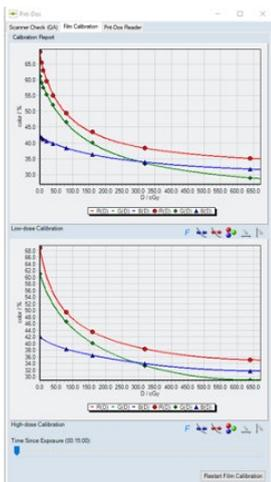
figure 5-6: low and high dose calibration curves
