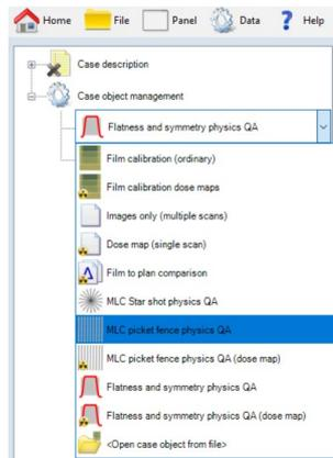
Click on "Add New Case Object" under the "Case Object Management" heading. A drop-down menu will appear and gives the user several options. Select "MLC Picket Fence Physics QA" (Shown left). Next, acquire the image by either reading it from a saved file or scanning it directly.
