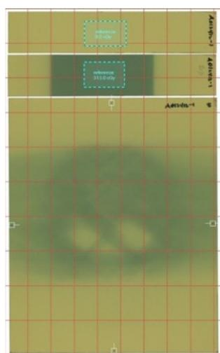
Here’s where the One Scan Protocol can be applied. Display the image of the application and reference films in the Image Panel and draw an area of interest on the unexposed reference strip. Then right click the region to designate it a calibration region and right click again on the frame to type in and enter the calibration value of zero. Notice that the frame changes color from yellow to blue to indicate it’s a
