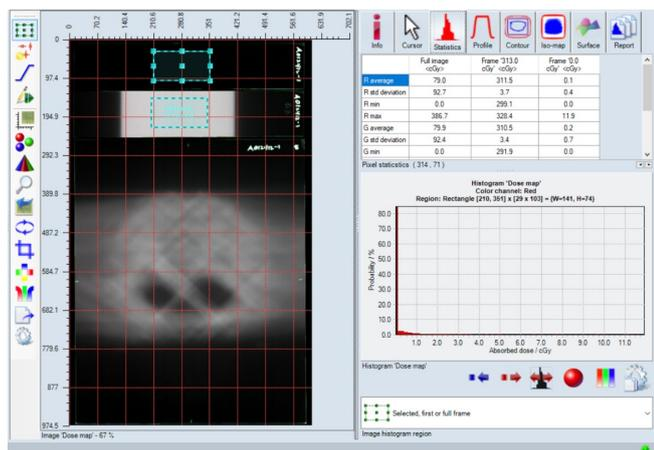
When FilmQA Pro™ software has finished calculating the dose map (using multi-channel dosimetry), select the dose map and draw areas of interest at the center of the two reference strips. Click the “Statistics” tab to show a table of dose values.
