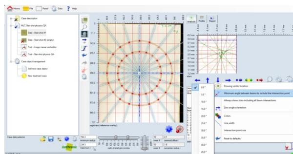
The result (Figure 10) shows that 27 of 35 intersection points were used. The radius of the minimum circle encompassing all intersections is reduced to 0.7 mm. The intersection-point centroid is still 0.8 mm from isocenter.
