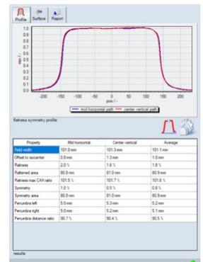
The profile data can be normalized in different ways. Use the Profile Normalization Tool
