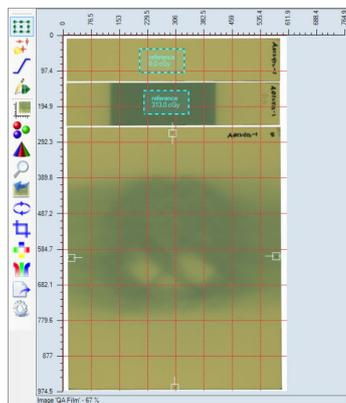
This efficient protocol was developed to simplify radiochromic film calibration and to avoid the complications of the post-exposure growth of radiochromic film response and the scan-to-scan variability of the scanner. The protocol provides a time-saving method for
