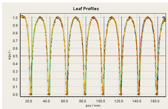
Truncate at smallest local minimum and maximum values and normalize to 0 and 1: Truncate lower part of the profile at highest minimum and upper part of the profile at lowest maximum and then normalize resulting profile to 0 and 1. This approach is very advantageous especially when the leaf openings vary over a wide range (i.e., the dose varies a lot between the leaf openings).
