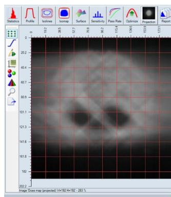
plan. The projection map is displayed in the projection tab. The projection map can be exported either as an image file or a CSV table to other applications. Icons along the left-hand border of the window give access to tools available in the Image Panel and described in that section.
