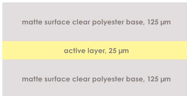
figure 1. structure of Gafchromic™ EBT-XD dosimetry film
