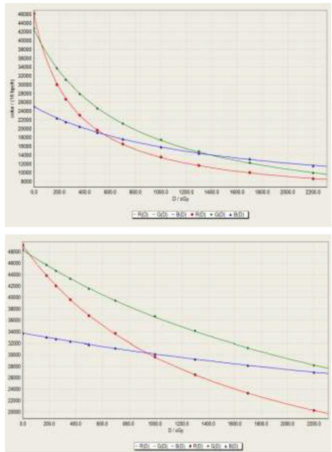
figure 2. Comparison of Calibration Curves of Gafchromic™ EBT3 (top) and EBT-XD (bottom) films
