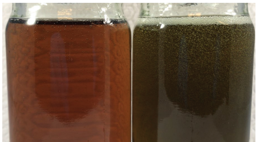
Figure 1: Comparison of foaming in promoted and initiated Derakane™ Signia™ 411 (left) and Derakane™ Momentum 411 (right) resin 1 minute and 30 seconds after initiation.
