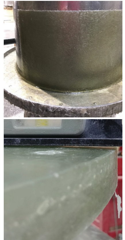
Figure 10: Derakane™ Signia™ 411 with CuNap manway on mold (top) and measure of flange drawback or curl after cure (bottom).
