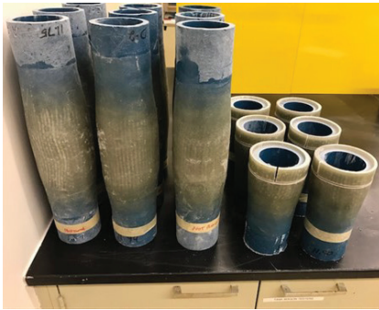
Figure 6. Preparation of M5 test specimens in a customer's shop (top) and precut and machined M5 test specimens (bottom).
