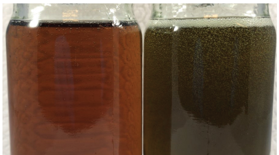
Figure 1: Comparison of foaming in promoted and initiated Derakane™ Signia™ 411 (left) and Derakane™ Momentum™ 411 (right) resin 90 seconds after initiation.
