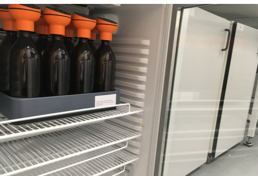
Respirometers for use in the OECD 301F methodology, an aerobic biodegradation test that determines the biodegradability of a material by measuring oxygen consumption.
