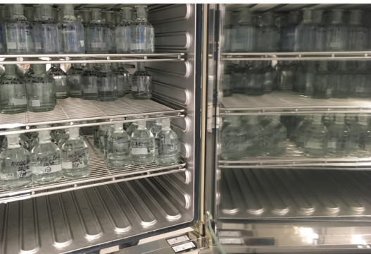
Biochemical Oxygen Demand (BOD) bottles in the incubator for use in the OECD 301D methodology, a respirometry test that predominantly measures biodegradation by dissolved oxygen and testing.
