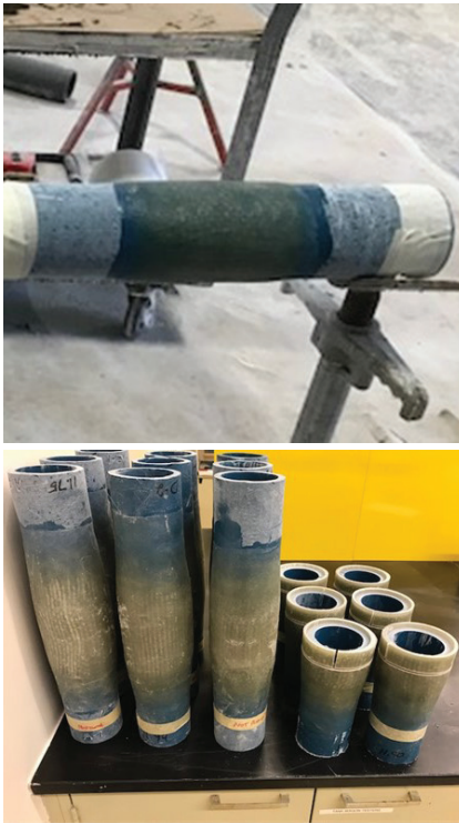
Figure 6. Preparation of M5 test specimens in a customer's shop (top) and pre-cut and machined M5 test specimens (bottom).
