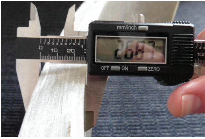
Figure 9: Measurement of thick filament wound tank section made in a single continuous step with Derakane™ Signia™ 411 resin.
