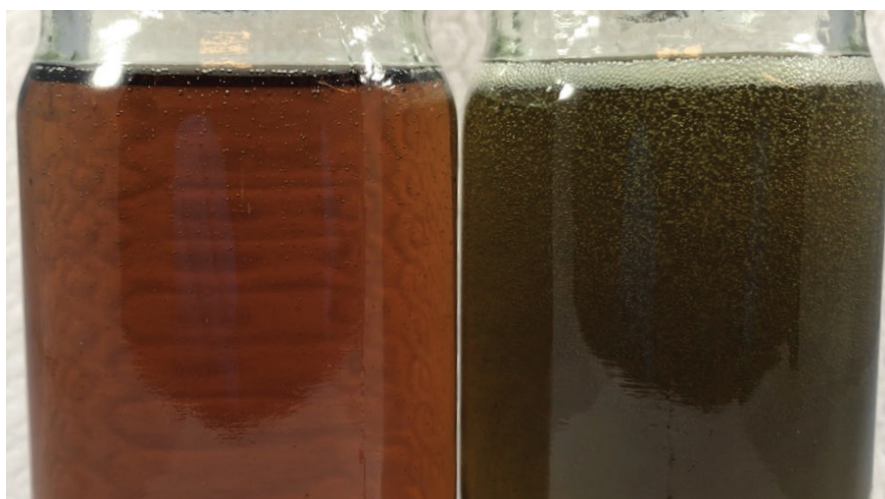
Figure 1: Comparison of foaming in promoted and initiated Derakane™ Signia™ 411 (left) and Derakane™ Momentum 411 (right) resin 1 minute and 30 seconds after initiation.
