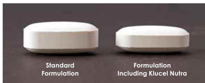
Figure 1. Lower binder use levels enable approximately 20% size reduction in final tablet size
